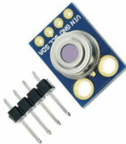
Fig. 6. The MLX90614 pins description
